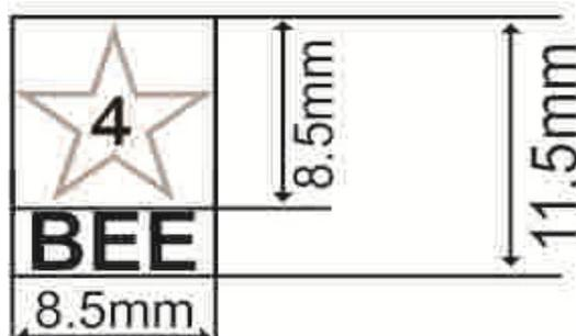
**Note:** The dimensions of label may be relatively reduced in accordance with the diameter of the tubular fluorescent lamp, provided the aspect ratio of the label shall remain the same.
