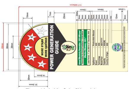
Figure 1 Label for Solar PV module
