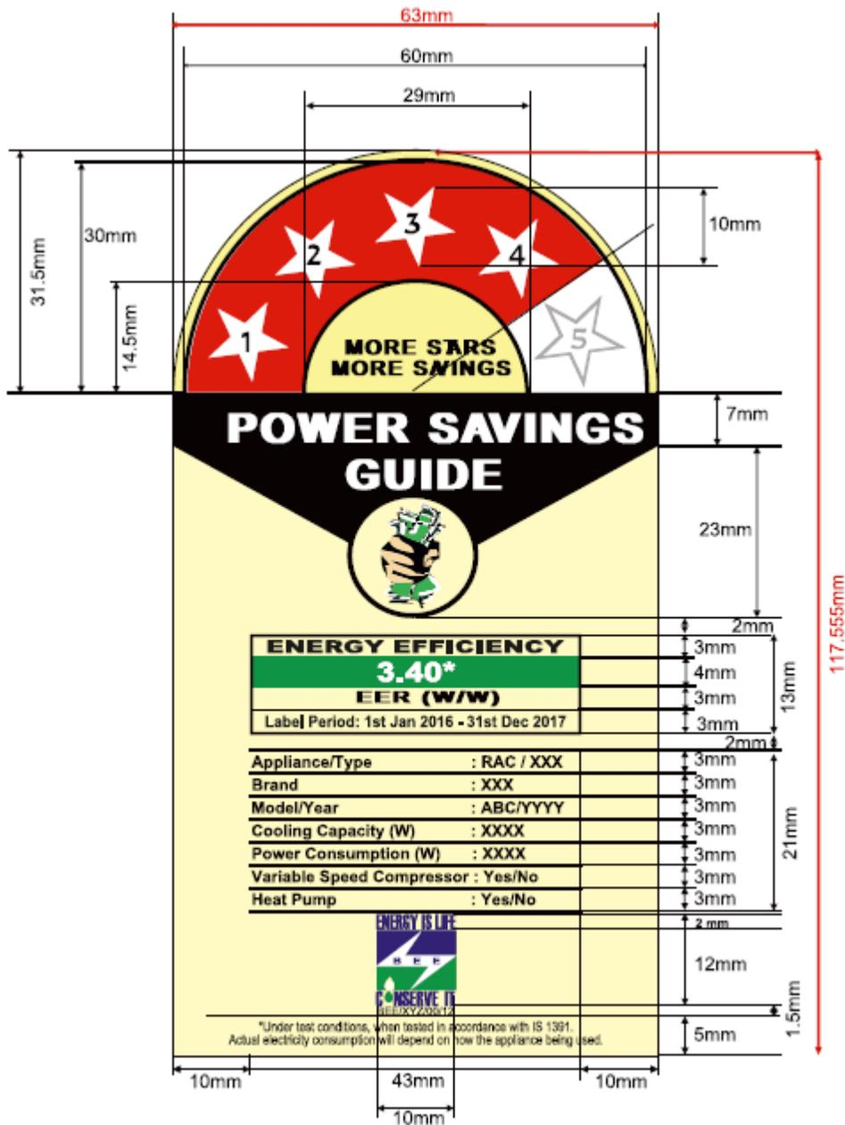
Figure 3.1: Design Scheme for the Label (Sample).
