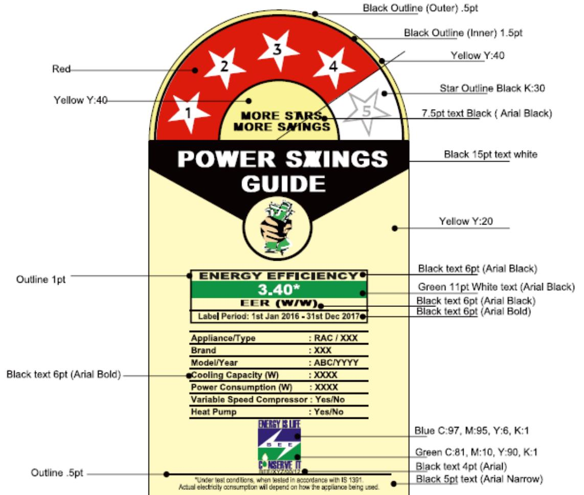
Figure 3.2: Colour Scheme for the Label (Sample).
